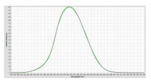
The f1' value, specified in percentage error, represents the degree to which the relative spectral responsivity deviates from the CIE V( $\lambda$ ) curve.
