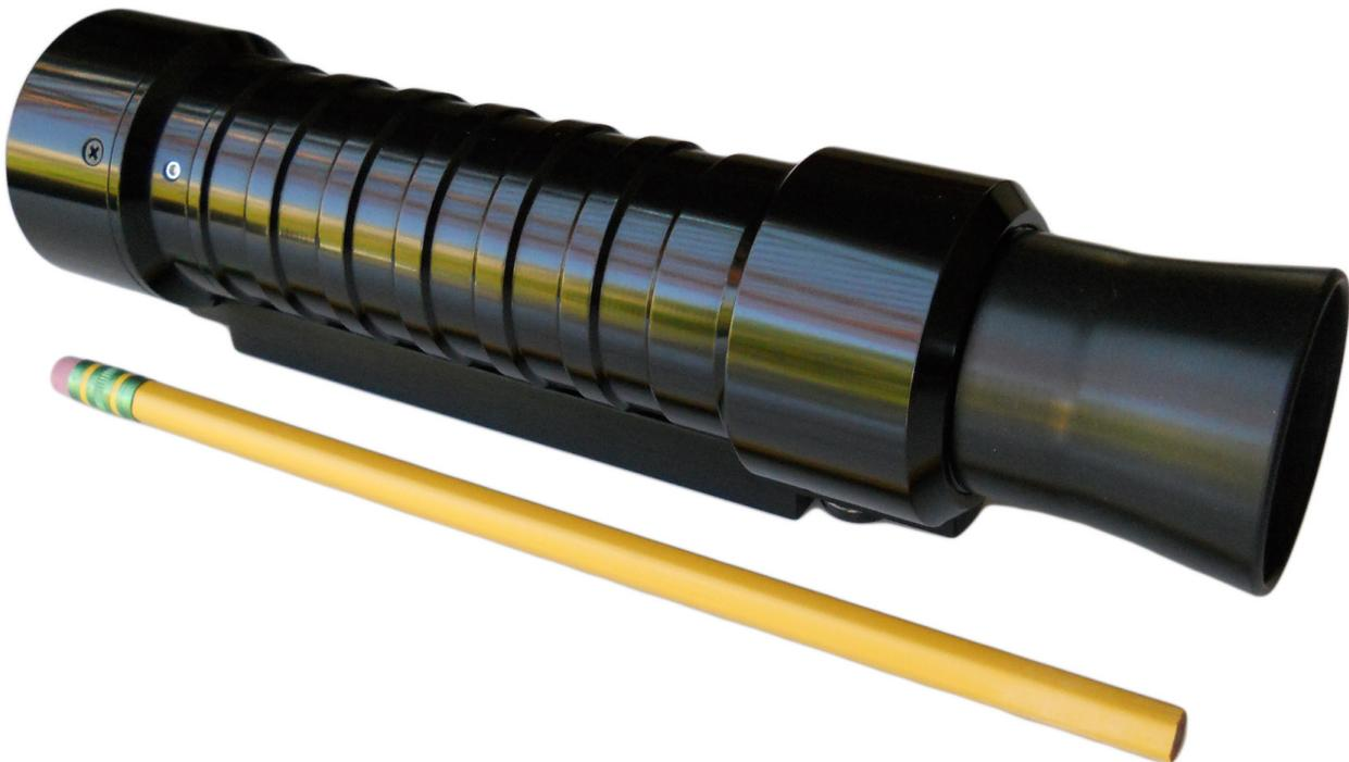
The CR-250-RH is a high resolution spectroradiometer/spectrophotometer in a very compact footprint with a 4 nm bandwidth and 1.6 nm/pixel resolution that excels in low-light, highly accurate wavelength and color measurements. It's ideal for measuring current and future display technologies as well as projectors including 6P projector technology.
